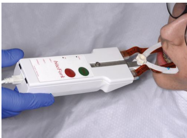
Figure 4: Bitefork System for bite force measurement. Maximum bilateral bite force at T1 ranged between 93.6N, left, and 104.8N right, in total, 198.4N.
